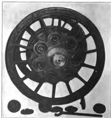
Fig. 4657. Driving Wheel with Caps Removed Showing Pockets for Driving Pins on Quill. Westinghouse A. C. Electric Locomotive.
